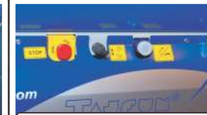
Controls for log loader or RN, conveyor belt; STOP function
