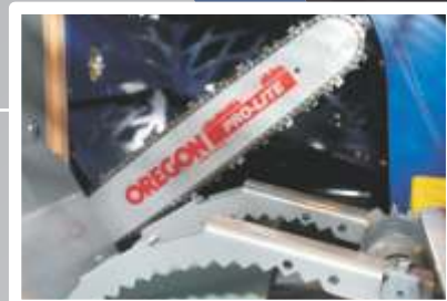
The chain saw With high cutting speed 25m/s (12.000 min -1 ) Cutting with the chain saw is quick and secure, the maintenance is easy.
