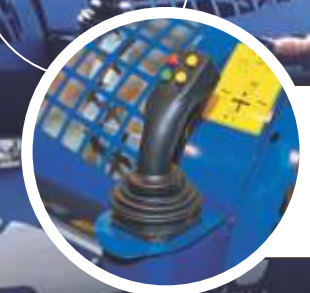
Joystick - ergonomic and simple control All basic function buttons of the machine (left and right loading, cutting, setting of the splitting wedge height, etc.) are located on one single control stick.
