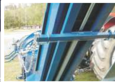
Discharge conveyor (4m): two stage telescope with automatic hydraulic belt straining. Continuous speed control of the conveyor belt. Adjustable conveyor speed button - on the operator's side Option-RCA 400 joy TG with the slewing discharge conveyor The conveyor has the possibility to move at an angle of 15° to the left and to the right, which enables filling of three pallets.
