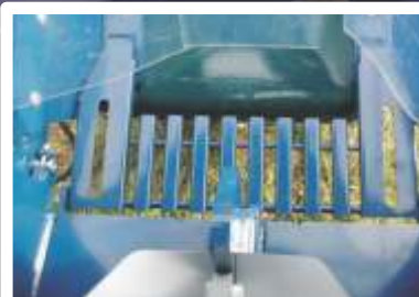
Lattice for sawdust between the splitting wedge and conveyor.
