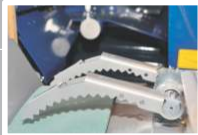
Hydraulic log holder With the log holder, the log is kept in the steady position and prevented from (over) turning, which also enables the right fall of the last piece into the splitting chute.
