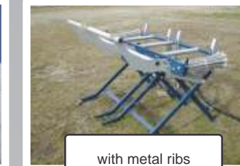
LOG LOADER DM 1511 is foldable and can be simply transported with the RCA Log lifting control - on the operator's side, Remote control - optional
