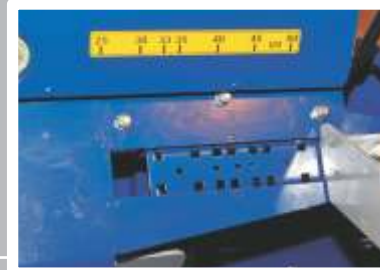
Hydraulic Length Limiter The length limiter is set from 25-50 cm at 5 cm stages.
